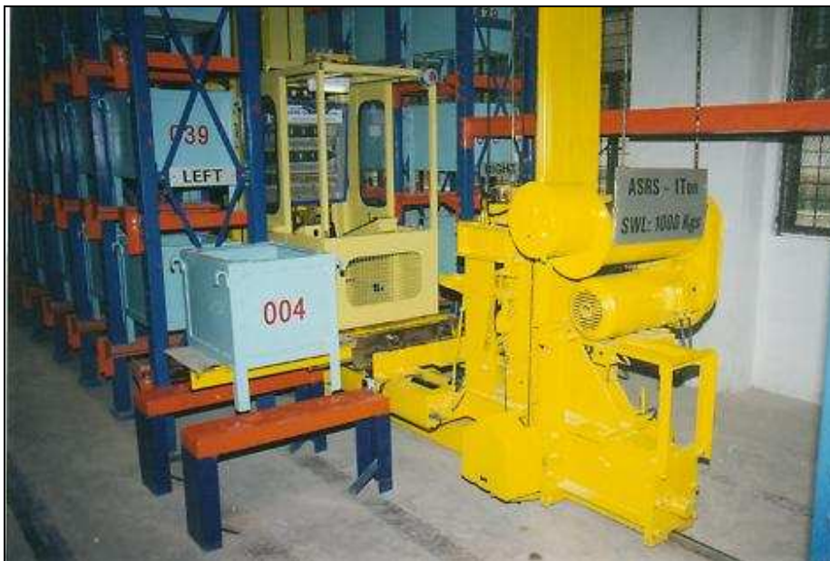
Figure 3: Crane with operator cabin at the background
