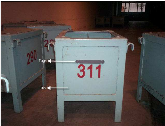
Figure 2: Metallic bin with RFID tag
