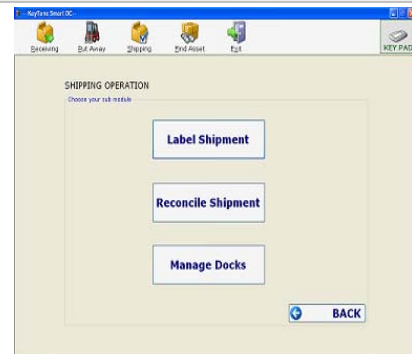
Operator interface to create RFID shipping labels, perform order verification and dock management
